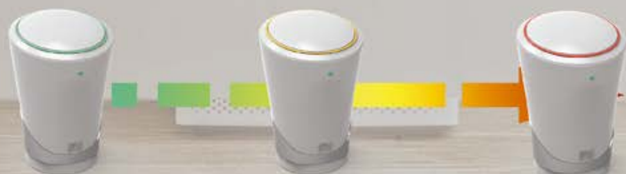
The light color change at the top of the lid indicates how much garbage inside bucket capacity
